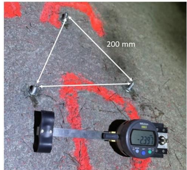
Fig. 6 A triangular setup of studs was used to directly measure unrestrained shrinkage on sprayed concrete panels and restrained shrinkage on the rock wall.
