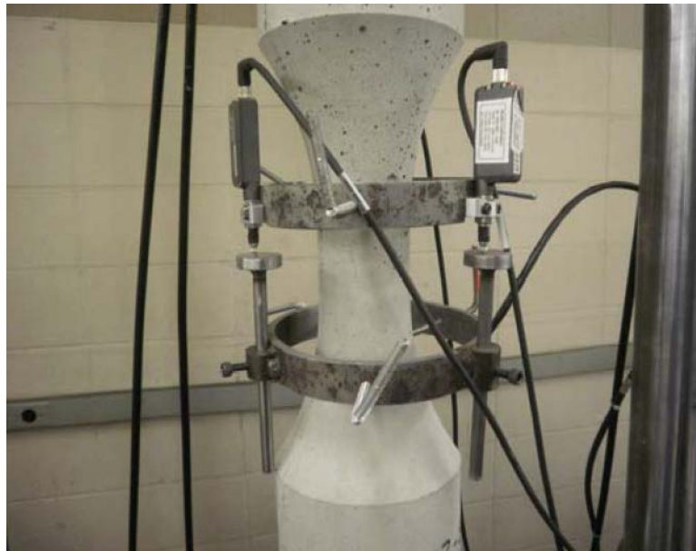
Figure 5: Direct Tensile Test Setup
