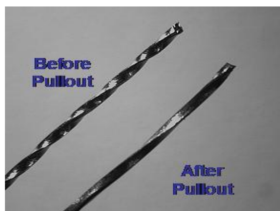
Figure 4: Twisted Steel Micro Reinforcement
