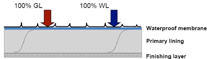
*Figure 9: Single Shell Lining with waterproof membrane*
