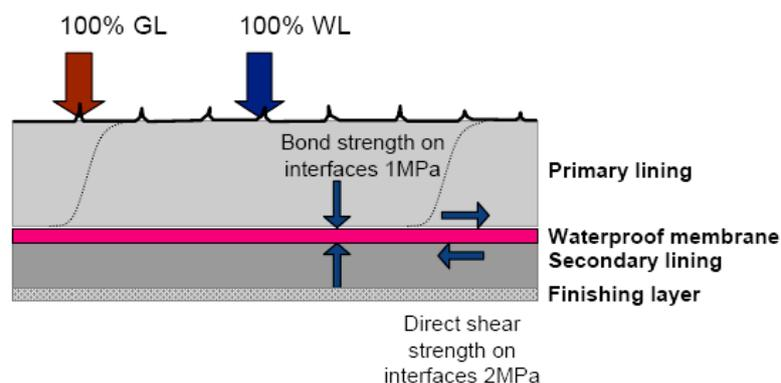
Figure 8: Fully Composite Shell Lining
