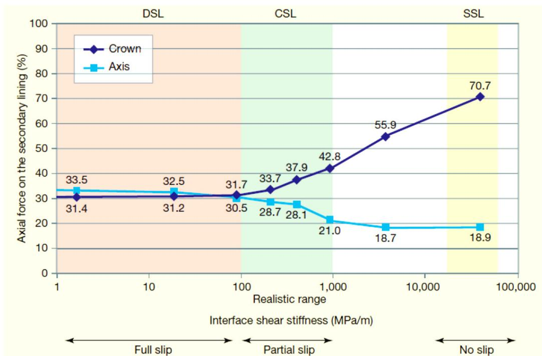
Figure 6: The hoop load in a secondary lining vs. the shear stiffness of the interface with the primary lining [9]
