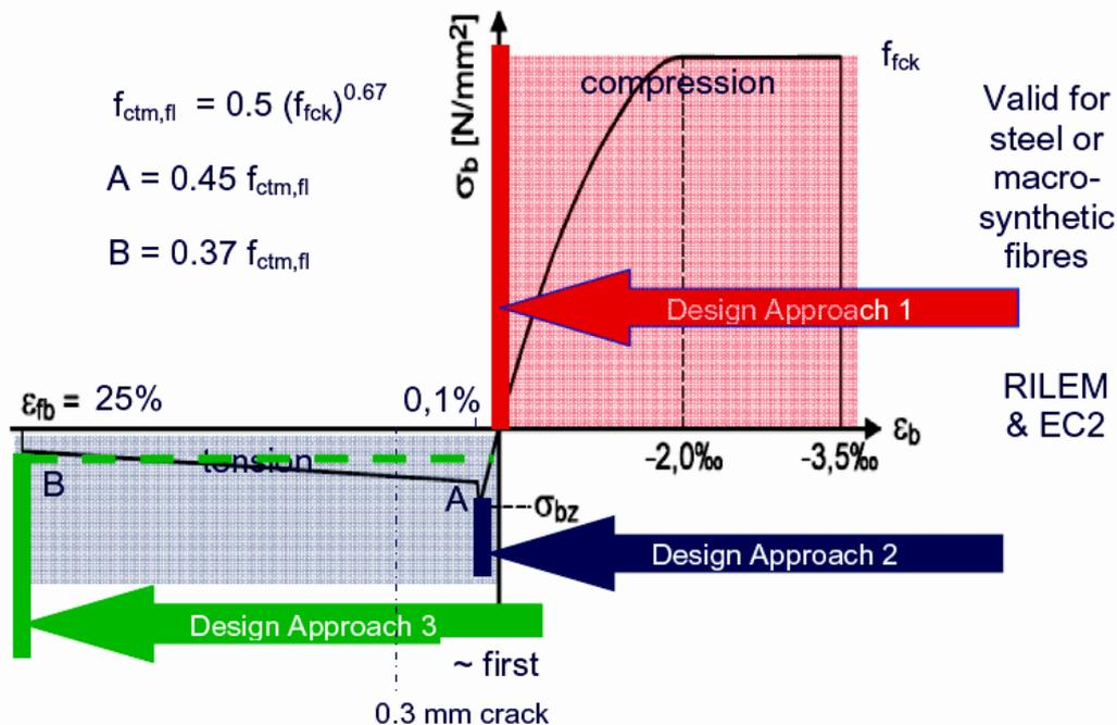
Figure 7: Simplified stress-strain models for fibre reinforced concrete
