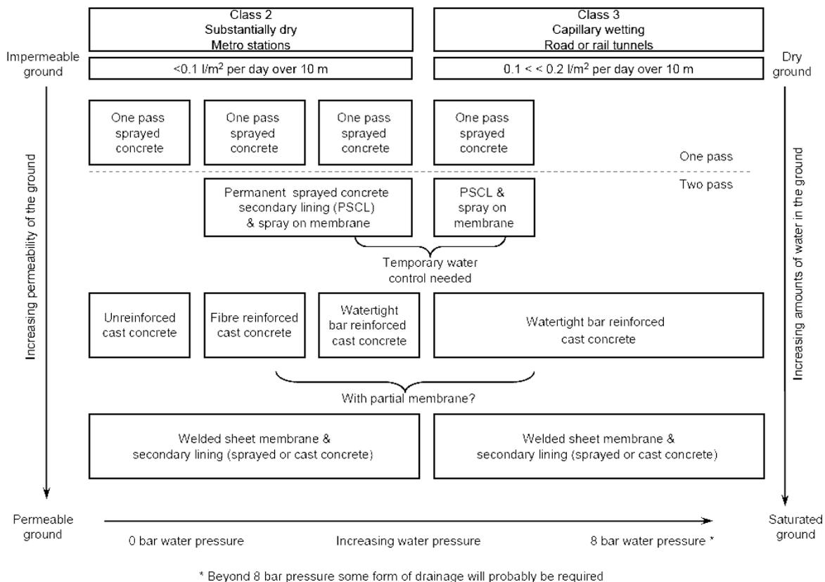
Figure 1: Design options for linings and waterproofing [1]
