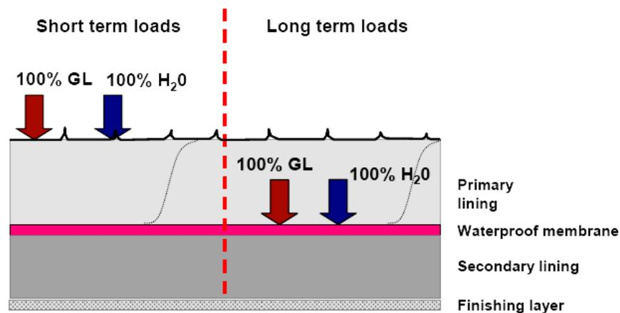
Figure 2: Typical Double Shell lining
