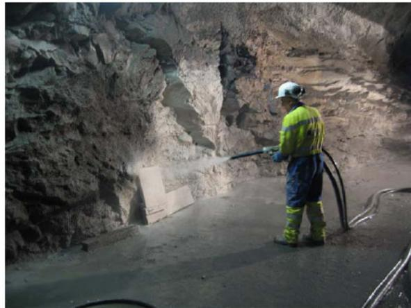
*Figure 13: Spraying TSL Meyco 865 onto a test panel, Hagerbach*
