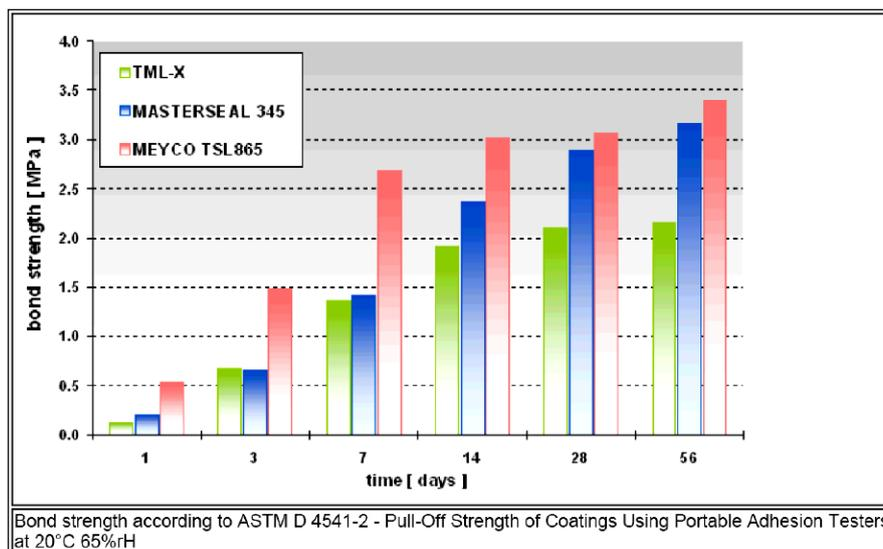
Figure 16: Bond strength vs. age under laboratory conditions
