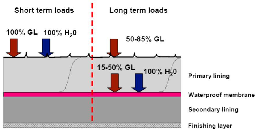
Figure 3: Typical Composite Shell Lining (partial composite with no shear or adhesive bond)
