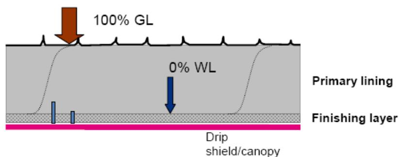
Figure 5: Typical Single Shell Lining
