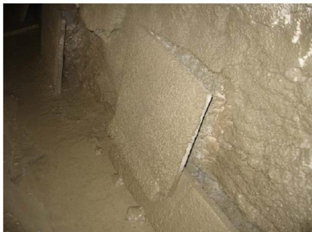
*Figure 14: Test panel: Sprayed concrete onto 30 minutes cured TSL Meyco 865*
