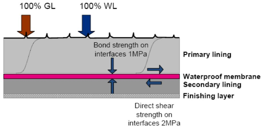
Figure 4: Fully Composite Shell Lining
