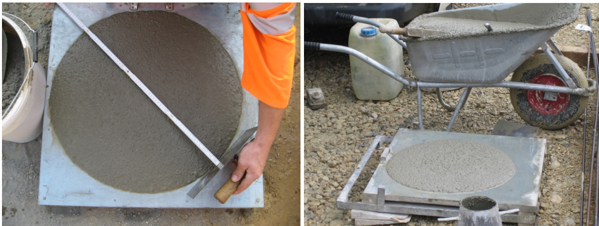
Figure 1: Slump of mixture 6 (left) and 6a (right)
