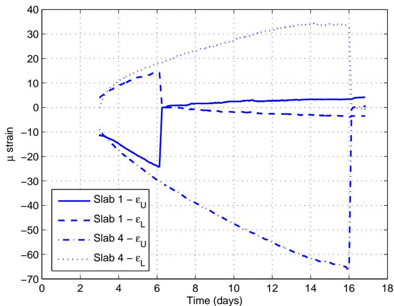
Figure 15: Measured strains for test slabs 1 (unreinforced) and 4 (reinforced), at upper (U) and lower (L) strain gauge positions. From [13].
