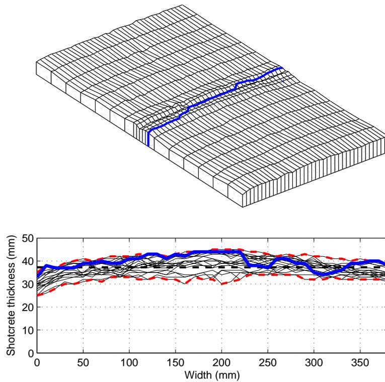
Figure 14: Surface profile and shotcrete thickness for glass fibre reinforced test slab (no. 4). Crack drawn with solid line, mean thickness with a straight dashed line. From [13].
