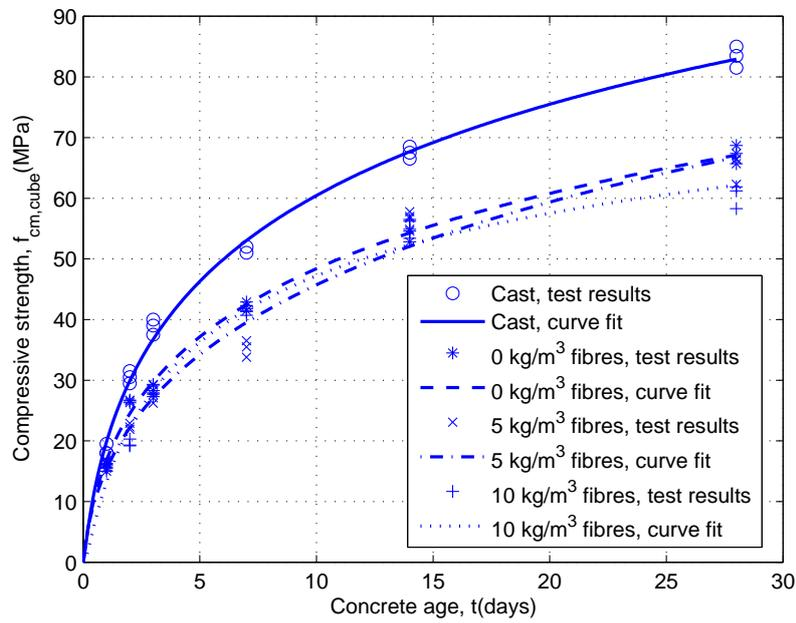
Figure 11: Compressive cube strengths for sprayed and cast reference samples. From [13].
