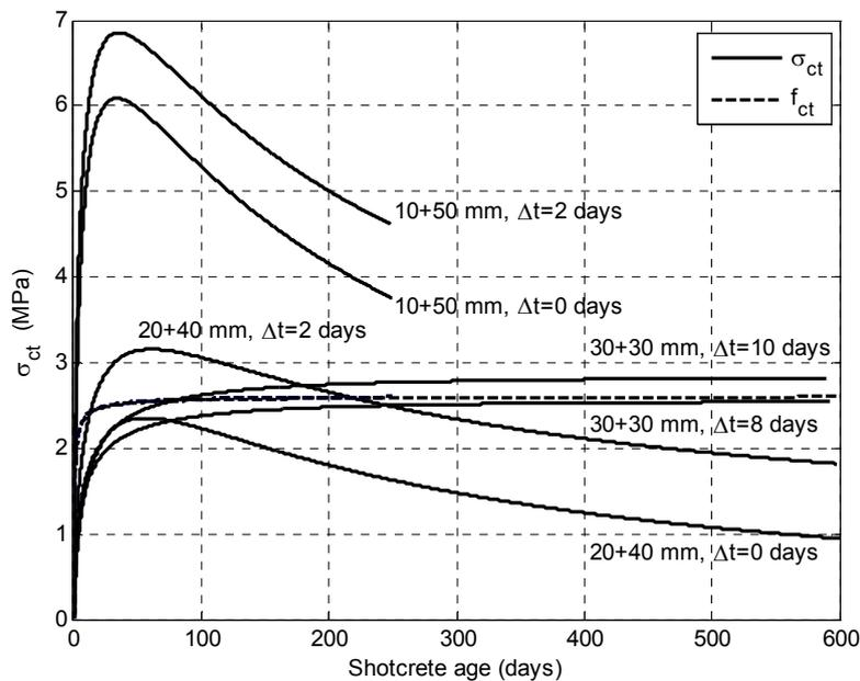
Figure 8: Shrinkage stresses in two-layer shotcrete beams at RH=75 %. The time between spraying and without watering is  $\Delta t$ . The outer layers are 10, 20 or 30 mm and the inner 50, 40 or 30 mm, respectively. From [6].
