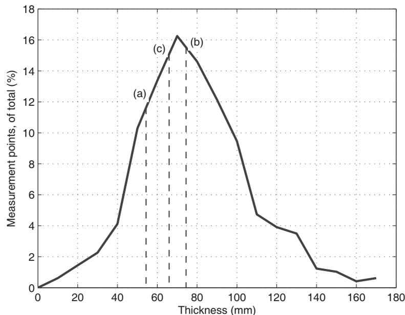
Figure 4: Shotcrete thickness measured in the Southern Link tunnels. The average thicknesses for the three examples (a–c) in Figure 3 are indicated. From [6].
