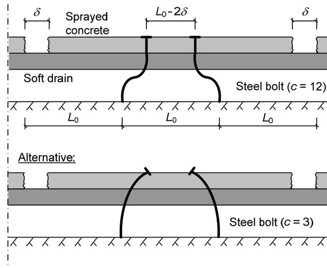
Figure 5: Shrinkage cracking of bolt anchored shotcrete on soft drains. Here  $c$  is a stiffness coefficient, depending on the connection between bolt and shotcrete. From [9].
