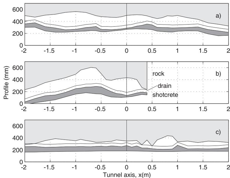
Figure 3: Three examples (a–c) of rock-drain-shotcrete (top to bottom) sections of 4 m length around cracks situated at  $x = 0$ . From [6].
