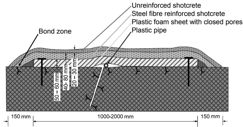
Figure 1: Shotcreted drain on rock – one strip of drain mat covering cracks in the rock. From [5].
