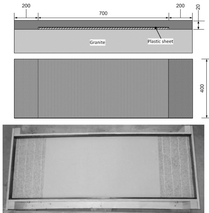
Figure 9: End-restrained shrinkage test specimen with 700 mm de-bonded length. From [13].
