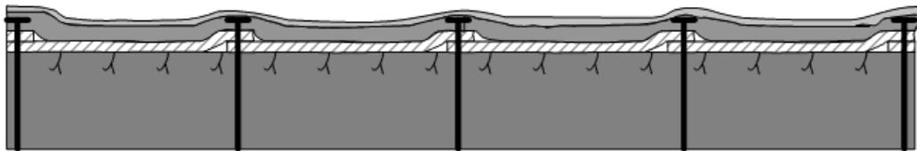
Figure 2: Section of shotcreted drains on rock. Two layers of shotcrete and steel bolts. From [6].
