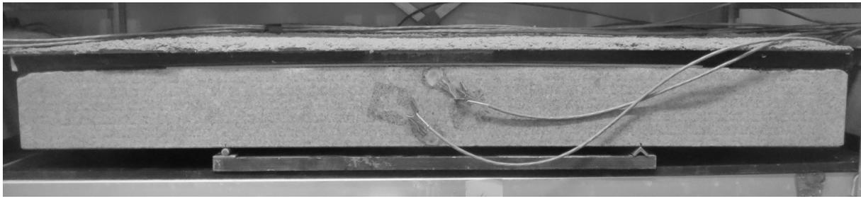
Figure 10: End-restrained test specimen, with shotcrete on granite slab with strain gauges. From [13].
