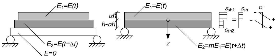
Figure 7: Models of a beam consisting of two shotcrete layers with different shrinkage. A 50 mm thick drain mat is included in the left model. From [6].
