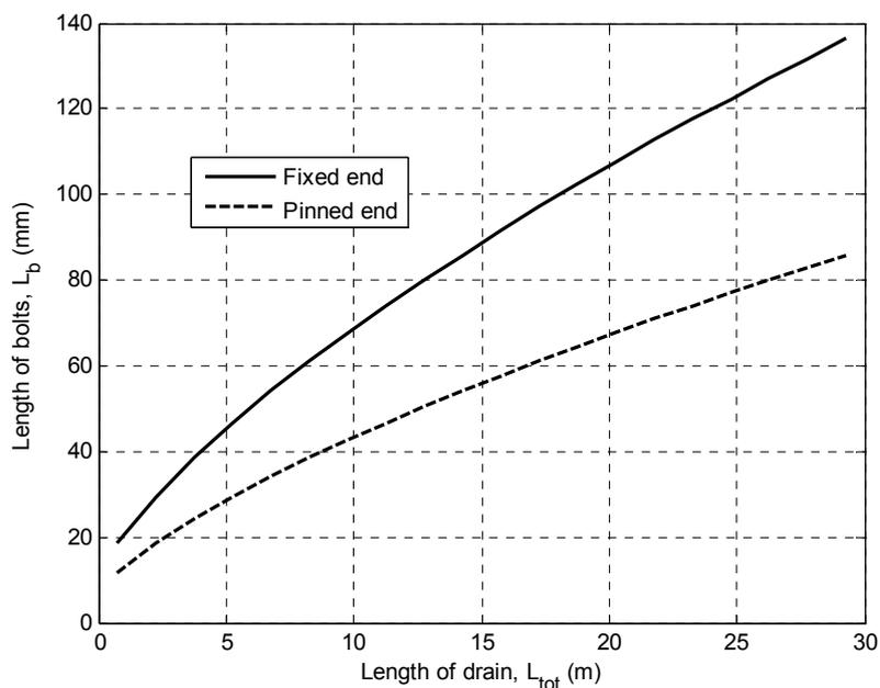
Figure 6: Relation between un-cracked length of shotcreted drain and length of anchoring steel bolts. From [9].
