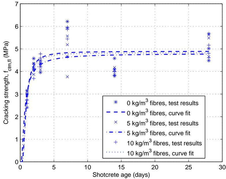
Figure 12: Flexural crack strengths from testing of shotcrete. From [13].
