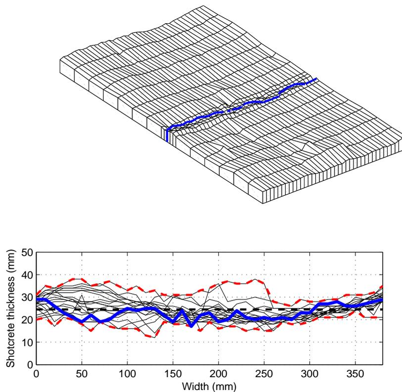
Figure 13: Surface profile and shotcrete thickness for unreinforced test slab (no. 1). Crack drawn with solid line, mean thickness with a straight dashed line. From [13].
