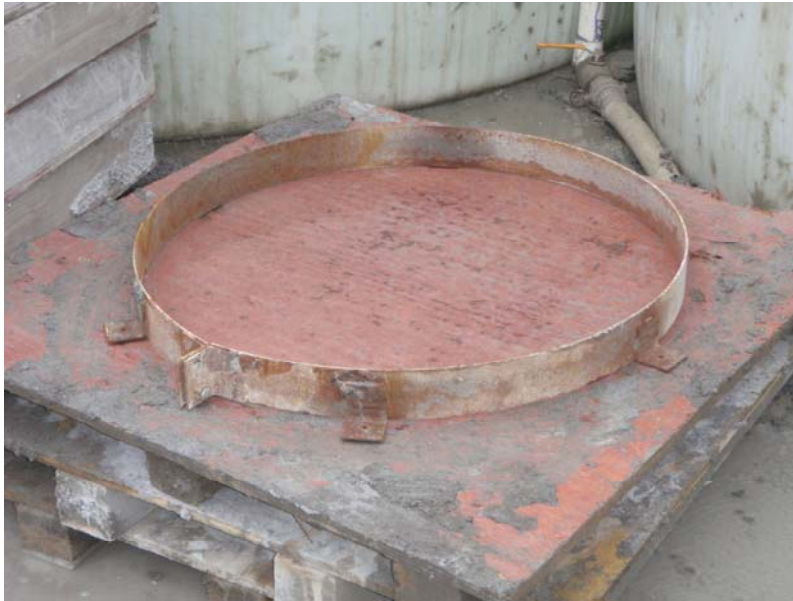
Figure 4: Metal form for panels mounted on wooden pallet (Picture: Jeramy Decker)
