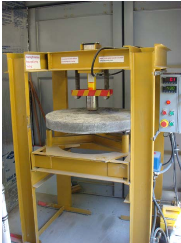
Figure 3: Round Determinate Panel Test machine with panel (Picture: Timothy O'Brien)
